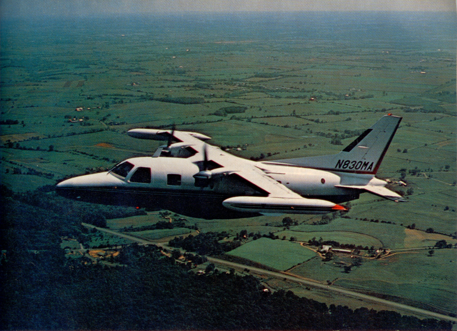
The MU-2L has long "legs." At 25,000 feet, maximum range, with 30 minutes' fuel reserve, is 1,450 statute miles; with 45 minutes' reserve, 1,380 statute miles. Photos by Berl Brechner.
