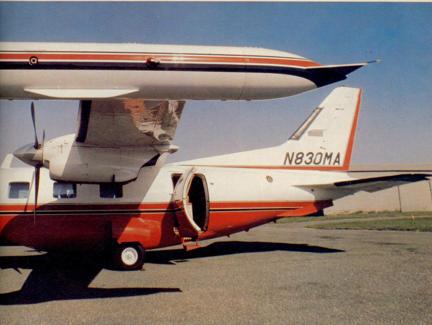
The airframe of the MU-2L has been structure tested for a service life of 25,000 flight hours. Engine time-between-overhauls is 3,000 flight hours.
