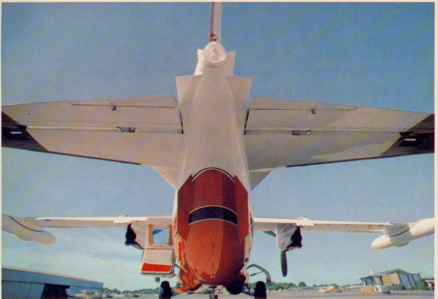
Two stabilizing fins are attached to the underside of the aft fuselage section to improve low-speed stability. Fiberglass reinforced plastic is used for tail cone, dorsal fin, and stabilizer tips.
